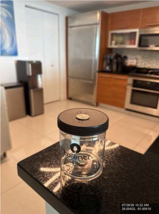
Photo 21 - Kitchen & Laundry - Freezer power outage indicator
